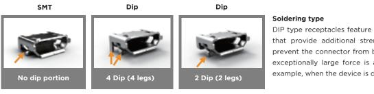
DIP type receptacles feature 2 or 4 through-hole solder legs that provide additional strength to the connector. They prevent the connector from being ripped off the board if an exceptionally large force is applied to the connector (for example, when the device is dropped with an inserted plug).
