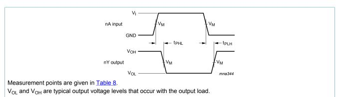
Figure 8. nA input to nY output propagation delays
