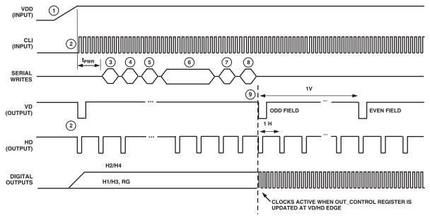
Figure 14. Recommended Power-Up Sequence
