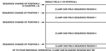
UP TO FOUR INDIVIDUAL HORIZONTAL CLAMP AND BLANKING REGIONS MAY BE PROGRAMMED WITHIN A SINGLE FIELD, USING THE SEQUENCE CHANGE POSITIONS.
