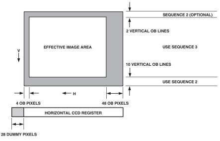
Figure 24. Example CCD Configuration
