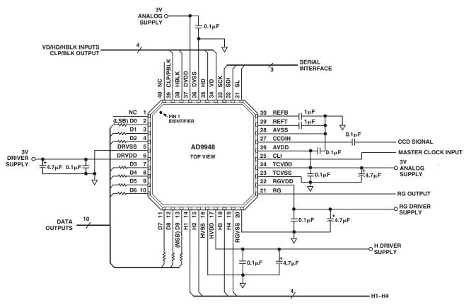
Figure 21. Recommended Circuit Configuration
