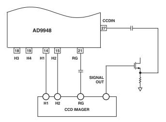
Figure 22a. CCD Connections (2 H-Clock)
