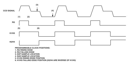
Figure 5. High Speed Clock Programmable Locations
