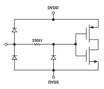
Circuit 4. Digital Inputs (Pins 31-35, 38)
