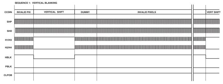
Figure 25. Horizontal Sequence during Vertical Blanking
