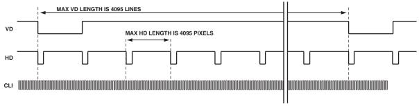
Figure 2b. Maximum VD/HD Dimensions
