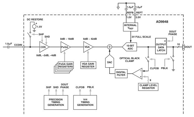
Figure 15. Analog Front End Functional Block Diagram
