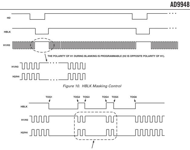
SPECIAL H-BLANK PATTERN IS CREATED USING MULTIPLE HBLK TOGGLE POSITIONS.
