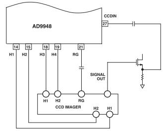
Figure 22b. CCD Connections (4 H-Clock)
