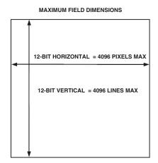
Figure 2a. Vertical and Horizontal Counters
