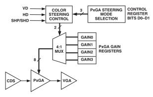
Figure 16. PxGA Block Diagram
