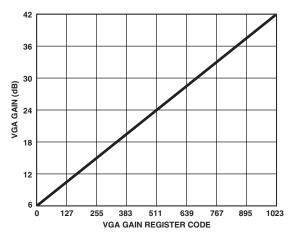
Figure 20. VGA Gain Curve (PxGA Not Included)
