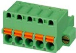
PCB connector, nominal current: 11 A, rated voltage (III/2): 320 V, number of positions: 5, pitch: 5.08 mm, connection method: Push-in spring connection, color: green, contact surface: Tin, The current, voltage and conductor cross section data refer to EU type-examination certificate No. KEMA 99ATEX3508U. The Ex rating is only valid in connection with ground terminal block ZFKK 1,5-MSTBV-5,08-PE/F-EX, order no. 1903232
