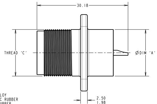
SPECIFICATIONS: MATERIAL: SHELL = ALUMINIUM ALLOY INSULATOR = SYNTHETIC RUBBER GASKET = SYNTHETIC RUBBER CONTACT = COPPER ALLOY FINISH:
