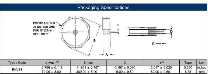
Dimension "E": This is a non-critical dimension that does not have a tolerance in the standard.
