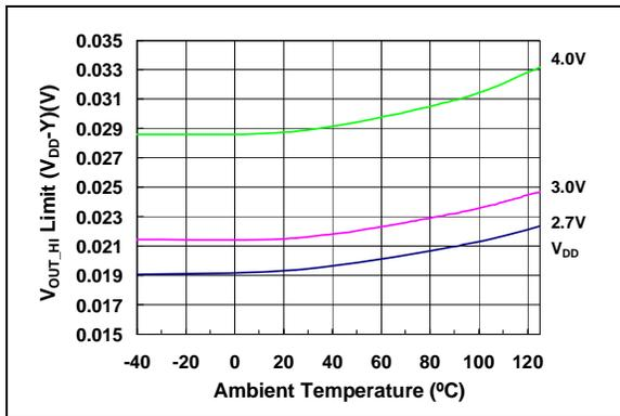
**FIGURE 2-25:**  *$V_{OUT}$  High Limit vs. Temperature and  $V_{DD}$ .*
