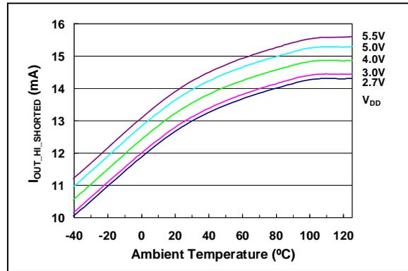
**FIGURE 2-27:**  *$I_{OUT}$  High Short vs. Temperature and  $V_{DD}$ .*
