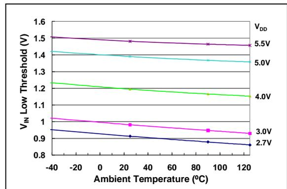
**FIGURE 2-23:**  $V_{IN}$  Low Threshold vs. Temperature and  $V_{DD}$ .
