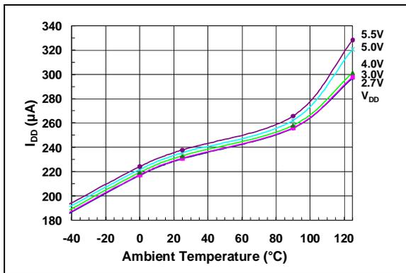
**FIGURE 2-15:**  $I_{DD}$  vs. Temperature and  $V_{DD}$ .
