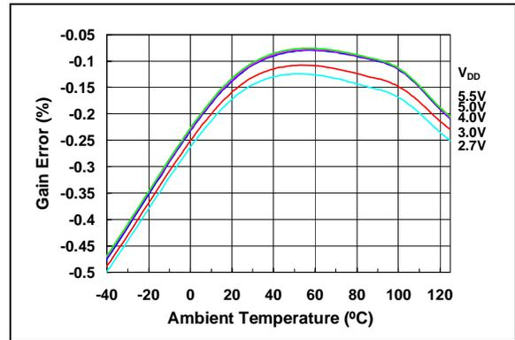
**FIGURE 2-21:** Gain Error vs. Temperature and  $V_{DD}$ .
