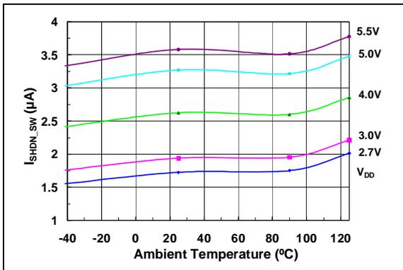
**FIGURE 2-19:** Software Shutdown Current vs. Temperature and  $V_{DD}$ .
