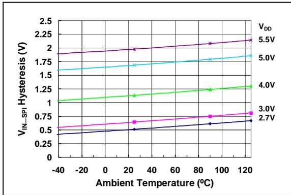
**FIGURE 2-24:** *Input Hysteresis vs. Temperature and  $V_{DD}$ .*
