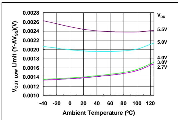
**FIGURE 2-26:**  *$V_{OUT}$  Low Limit vs. Temperature and  $V_{DD}$ .*
