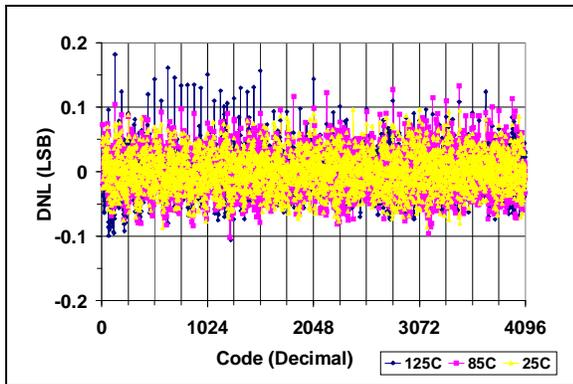
**FIGURE 2-2:** DNL vs. Code and Temperature (MCP4821).
