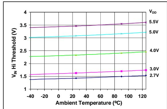
**FIGURE 2-22:**  $V_{IN}$  High Threshold vs. Temperature and  $V_{DD}$ .
