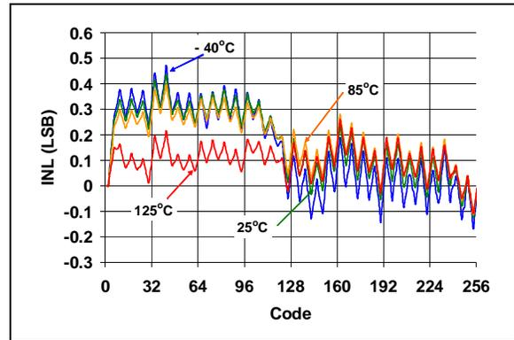
**FIGURE 2-10:** INL vs. Code and Temperature (MCP4801).
