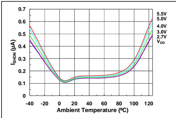
**FIGURE 2-18:** Hardware Shutdown Current vs. Temperature and  $V_{DD}$ .
