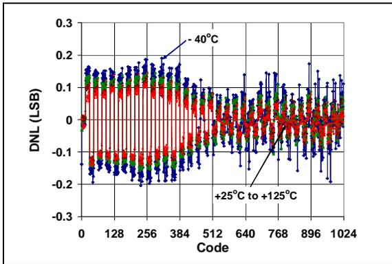
**FIGURE 2-7:** DNL vs. Code and Temperature (MCP4811).
