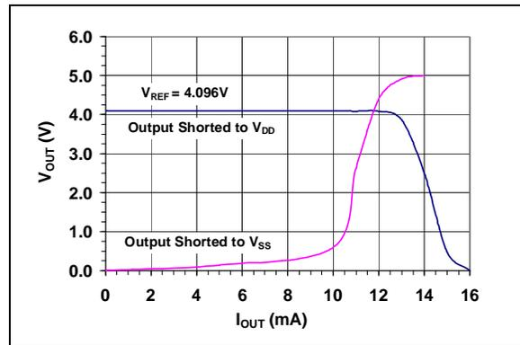
**FIGURE 2-28:**  *$I_{OUT}$  vs.  $V_{OUT}$ . Gain = 2x.*
