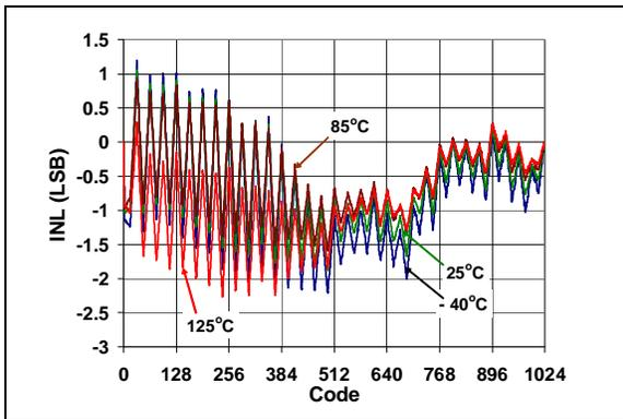
**FIGURE 2-8:** INL vs. Code and Temperature (MCP4811).
