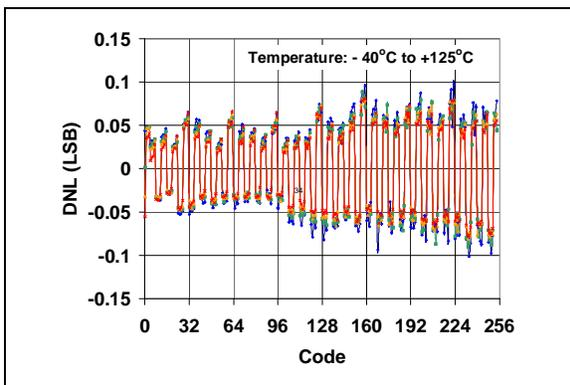
**FIGURE 2-9:** DNL vs. Code and Temperature (MCP4801).
