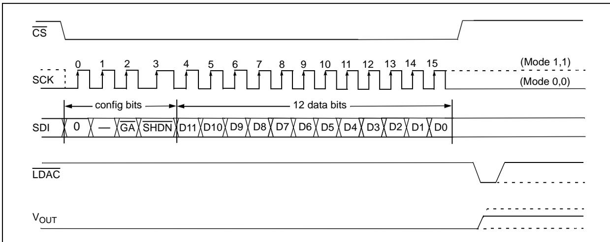
**FIGURE 5-1:** Write Command for MCP4821 (12-bit DAC).
