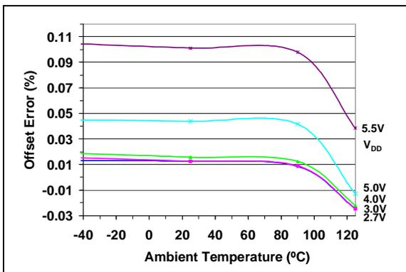
**FIGURE 2-20:** Offset Error vs. Temperature and  $V_{DD}$ .
