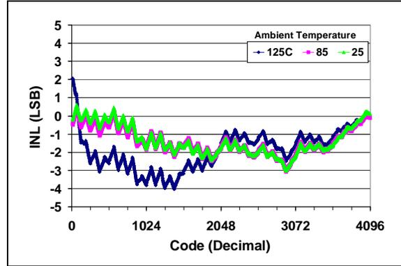
**FIGURE 2-4:** INL vs. Code and Temperature (MCP4821).
