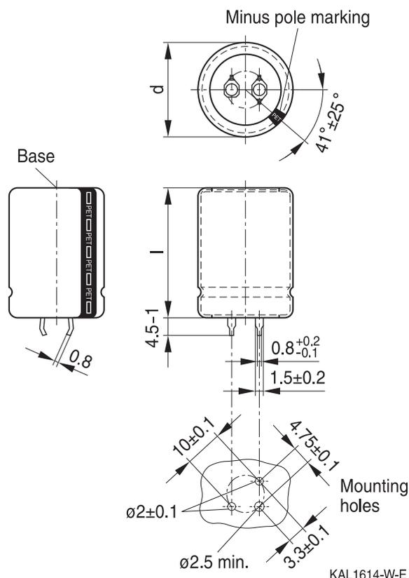
Snap-in capacitors are also available with 3 terminals (length ( $4.5 - 1$ ) mm). PET insulation is marked with "PET" on the sleeve. Safety vent on the case wall.
