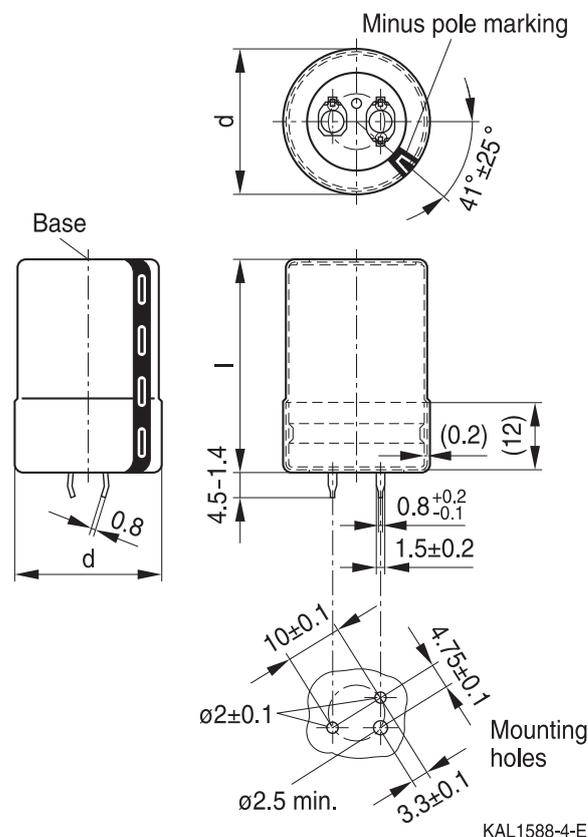
Snap-in terminals, length (6.3 +1/–1.4) mm. Also available in a shorter version with a length of (4.5 –1.4) mm. PET insulation cap is positioned under the insulation sleeve. Safety vent on the case wall.
