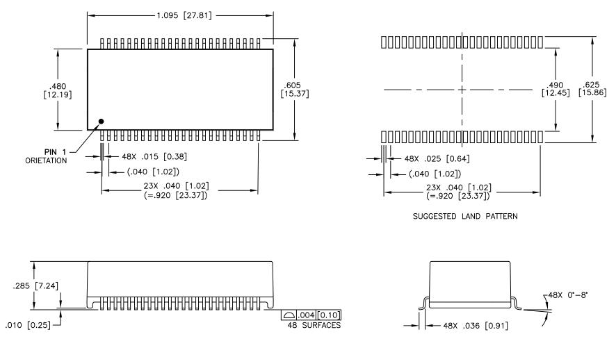
DIMENSIONS ARE IN INCHES [MILLIMETERS] WITH THE FOLLOWING TOLERANCES: [MILLIMETERS] ARE FOR REFERENCE ONLY. .XX=  $\pm$ .02 [ $\pm$ 0.5] .XXX=  $\pm$ .010 [ $\pm$ 0.25]
