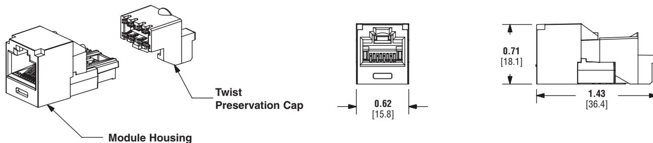
Dimensions are in inches [Dimensions in brackets are metric]
