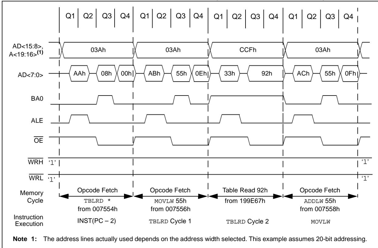
**FIGURE 7-9: EXTERNAL BUS TIMING FOR TBLRD (EXTENDED MICROCONTROLLER MODE)**
