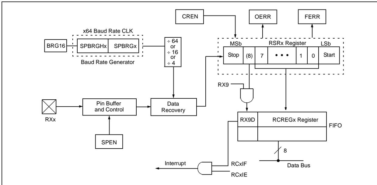
**FIGURE 20-7: ASYNCHRONOUS RECEPTION**
