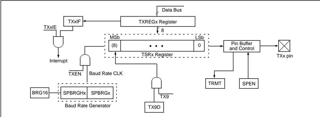
**FIGURE 20-4: ASYNCHRONOUS TRANSMISSION**
