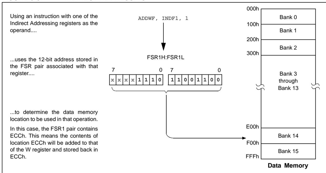
The PLUSW register can be used to implement a form of Indexed Addressing in the data memory space. By manipulating the value in the W register, users can reach addresses that are fixed offsets from pointer addresses. In some applications, this can be used to implement some powerful program control structure, such as software stacks, inside of data memory.
