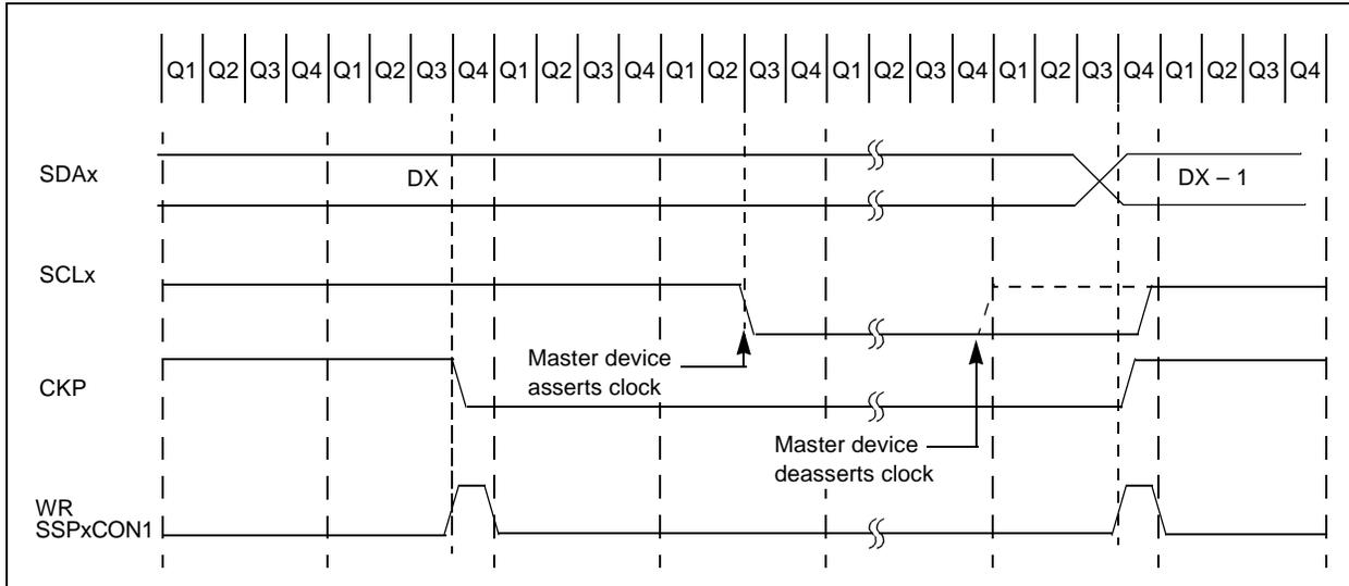
**FIGURE 19-13: I<sup>2</sup>C™ SLAVE MODE TIMING WITH SEN = 1 (RECEPTION, 7-BIT ADDRESS)**
