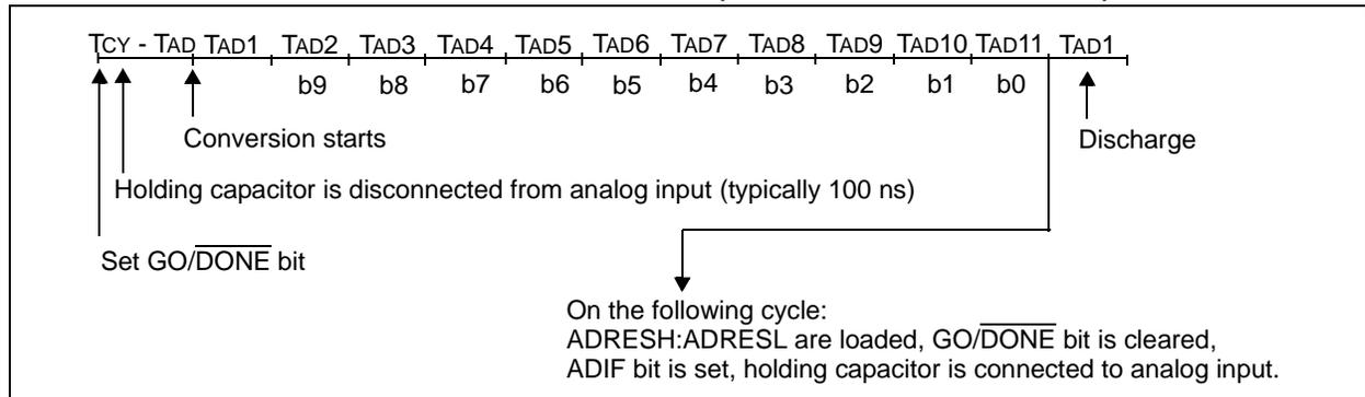
**FIGURE 21-5: A/D CONVERSION TAD CYCLES ( $\text{ACQT}\langle 2:0 \rangle = 010, \text{TACQ} = 4 \text{ TAD}$ )**
