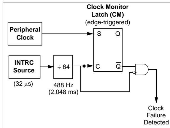
Clock failure is tested for on the falling edge of the sample clock. If a sample clock falling edge occurs while CM is still set, a clock failure has been detected (Figure 25-4). This causes the following:
