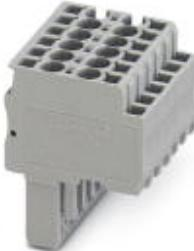
Plug, Connection method: Spring-cage connection, Number of positions: 13, Cross section: 0.08 mm<sup>2</sup> - 4 mm<sup>2</sup>, AWG: 28 - 12, Width: 67.6 mm, Height: 39 mm, Color: gray
