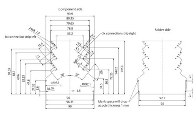
non dimensioned radii max R1 inhibited surface
