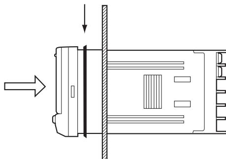
3. Fit the adaptor into the grooves on the left and right sides of the rear case, then push it until it contacts the panel to secure the K3MA-F.
