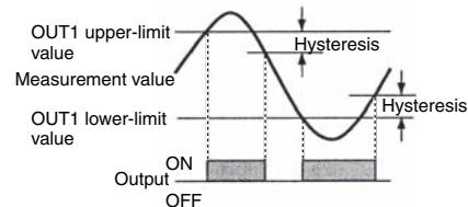
The three types of output operations shown above can be combined as desired. The following are examples of possible combinations.
