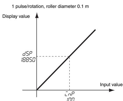
When displaying a flowrate (e.g., in  $\text{m}^3/\text{min}$  or  $\text{m}^3/\text{h}$ ), make the scaling settings after confirming the I/O characteristics of the flowrate sensor. There are flowrate sensors that output analog signals. If this kind of flowrate sensor is used, consider using the K3MA-J.
