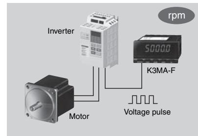
Note: If the monitor output from the inverter is analog, such as 0 to 10 V, use the K3MA-J.
