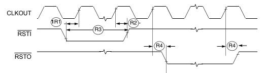
Figure 12. RSTI and Configuration Override Timing
