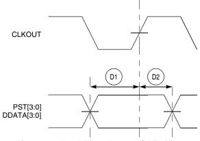
Figure 20. Real-Time Trace AC Timing
