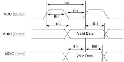
Figure 10. MII Serial Management Channel Timing Diagram
