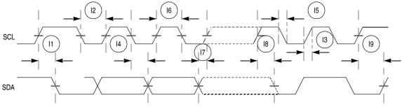
Figure 13. I2C Input/Output Timings
