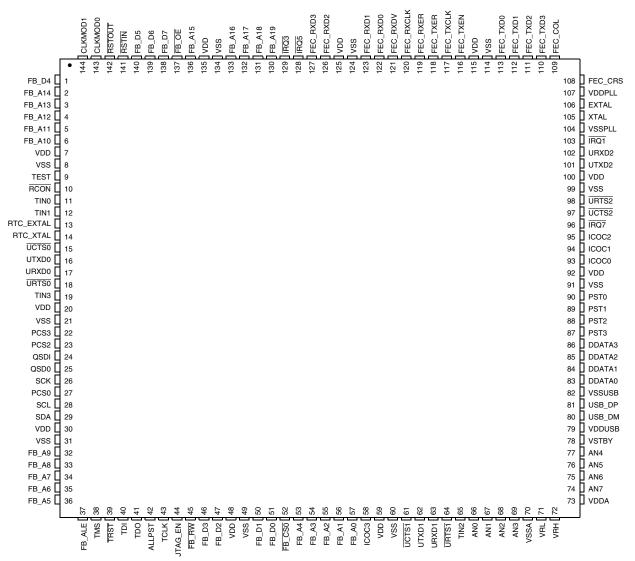
Figure 2. 144 LQFP Pin Assignment
