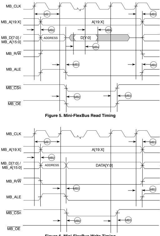
Figure 6. Mini-FlexBus Write Timing
