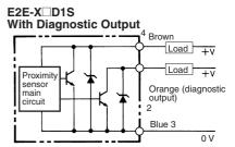
Note: Connect both the loads to the +V side of the control output and diagnostic output.
