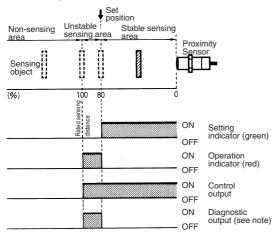
**lote:** The diagnostic output of the E2E-X□D1S is ON when there is a coil burnout or the sensing object is located in the unstable sensing range for 0.3 s or more.
