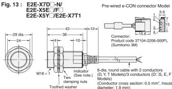
Note: D, T Models: Operation indicator (red), setting indicator (green); E, F, Y Models: Operation indicator (red)
