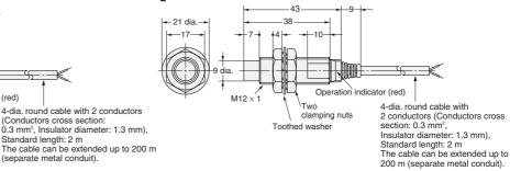
←21 dia.-+10 Indicator (See note.) Two 4-dia, cable with 2 conductors clamping nuts 4-dia. cable with 2 conductors (Conductors cross section: 0.3 mm², Insulator diameter: 1.3 mm), Standard length: 2 m
