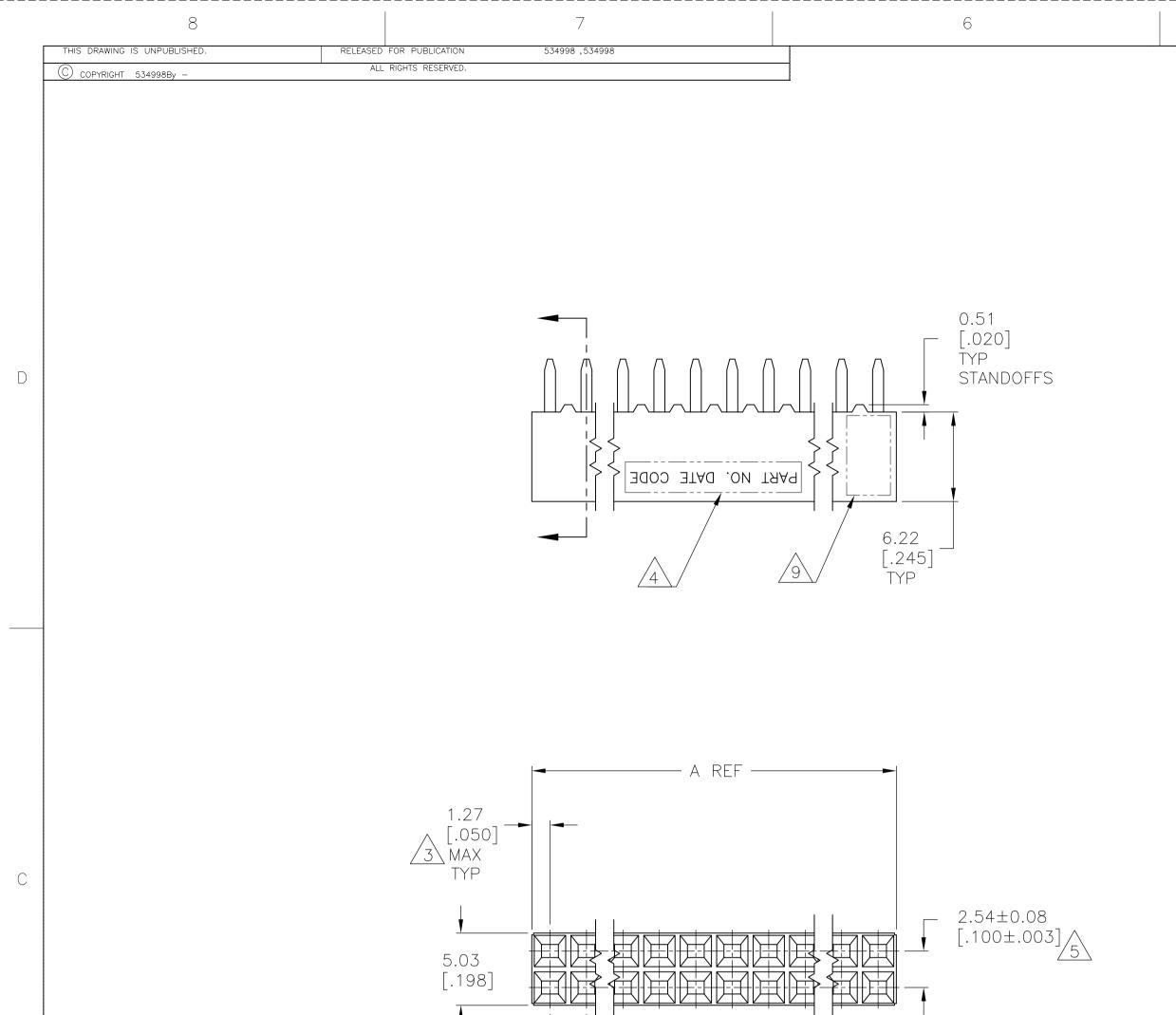
HOUSING: FLAME RETARDANT, GLASS FILLED, THERMOPLASTIC, COLOR: BLACK. CONTACT: PHOSPHOR BRONZE 12CONTACT: DUPLEX PLATED 0.76µm[.000030] GOLD IN CONTACT AREA, 3.81—7.62µm[.000150—.000300] BRIGHT TIN—LEAD ON LEADS, ALL OVER 1.27µm[.000050] NICKEL 3 these dimensions pertain to cavitly centerlines only – not to contact locations 4PART NUMBER AND DATE CODE ARE MARKED IN APPROXIMATE LOCATION SHOWN, EITHER SIDE.  $\sqrt{5}$ TOLERANCE IS NON-CUMULATIVE.
