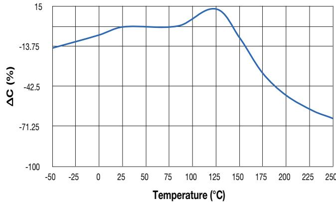
Typical Temperature Coefficient of Capacitance (COG Dielectric)
