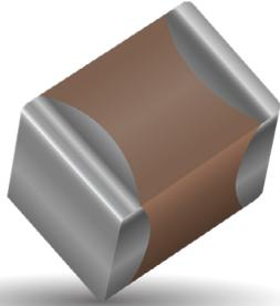
High value, low leakage and small size are difficult parameters to obtain in capacitors for high voltage systems. AVX special high voltage MLC chip capacitors meet these performance characteristics and are designed for applications such as snubbers in high frequency power converters, resonators in SMPS, and high voltage coupling/dc blocking. These high voltage chip designs exhibit low ESRs at high frequencies.
