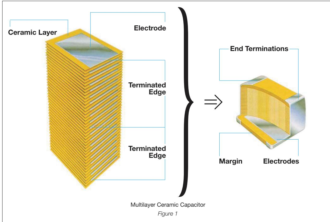
**Formulations** – Multilayer ceramic capacitors are available in both Class 1 and Class 2 formulations. Temperature compensating formulation are Class 1 and temperature stable and general application formulations are classified as Class 2.
