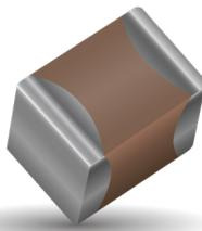
X7R formulations are called "temperature stable" ceramics and fall into EIA Class II materials. X7R is the most popular of these intermediate dielectric constant materials. Its temperature variation of capacitance is within  $\pm 15\%$  from  $-55^\circ\text{C}$  to  $+125^\circ\text{C}$ . This capacitance change is non-linear.
