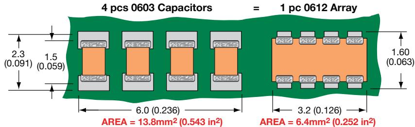
The 0612 4-element capacitor array gives a PCB space saving of over 50% vs four 0603 discretes and over 70% vs four 0805 discrete capacitors.
