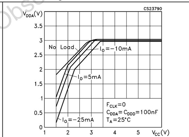
**Figure 7. Digital voltage regulator: line - load regulation**
