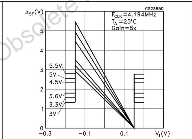
Figure 13. Gain response of  $\Delta\Sigma$  AD Converters
