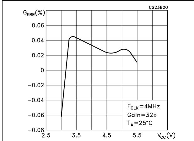
Figure 10. Power supply DC rejection vs.  $V_{CC}$
