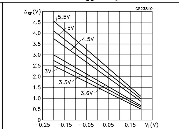
Figure 9. Power supply AC rejection vs.  $V_{CC}$
