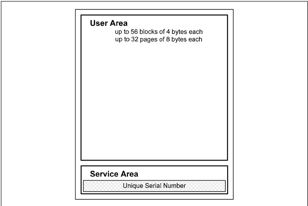
Figure 5: Memory principle of my-d<sup>®</sup> SRF 55V02P
