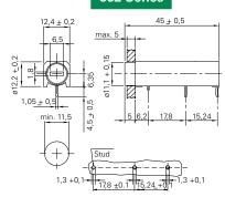
Holes in the printed circuit board: 1,3 +0,1
