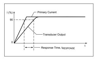
**Rise time** ( $t_r$ ). The time interval between a) when the sensor reaches 10% of its full-scale value, and b) when it reaches 90% of its full-scale value. The rise time to a step response is used to derive the bandwidth of the current sensor, in which  $f(-3 \text{ dB}) = 0.35/t_r$ . Both  $t_r$  and  $t_{RESPONSE}$  are detrimentally affected by eddy current losses observed in the conductive IC ground plane.
