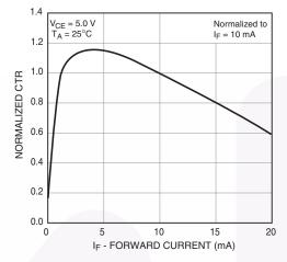
Fig. 3 Normalized CTR vs. Forward Current
