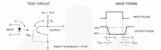
Figure 9. Switching Time Test Circuit and Waveforms
