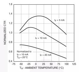
Fig. 4 Normalized CTR vs. Ambient Temperature
