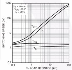
Fig. 6 Switching Speed vs. Load Resistor
