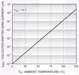
Fig. 5 Dark Current vs. Ambient Temperature
