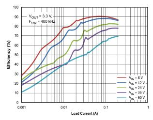
Figure 2. TPS54061EVM-142 Low Current Efficiency
