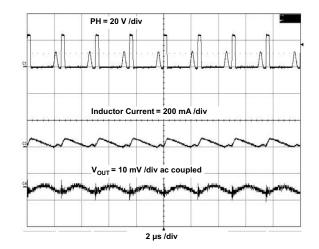
Figure 9. TPS54061EVM-142 Output Ripple DCM
