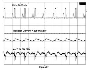
Figure 12. TPS54061EVM-142 Input Ripple DCM
