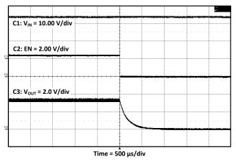
Figure 17. TPS54061EVM-142 Shutdown Relative to EN
