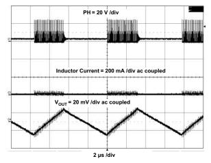
Figure 10. TPS54061EVM-142 Output Ripple Skip Mode
