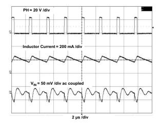
Figure 11. TPS54061EVM-142 Input Ripple CCM
