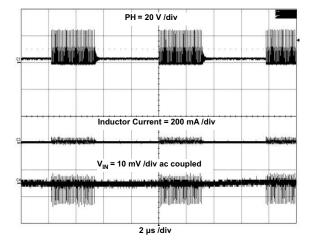
Figure 13. TPS54061EVM-142 Input-Ripple Skip Mode
