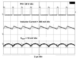
Figure 8. TPS54061EVM-142 Output Ripple CCM
