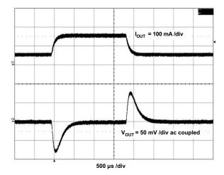
Figure 5. TPS54061EVM-142 Load Transient Response
