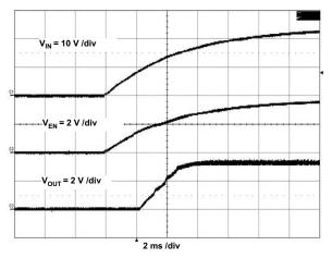
Figure 14. TPS54061EVM-142 Start-Up Relative to V<sub>IN</sub>
