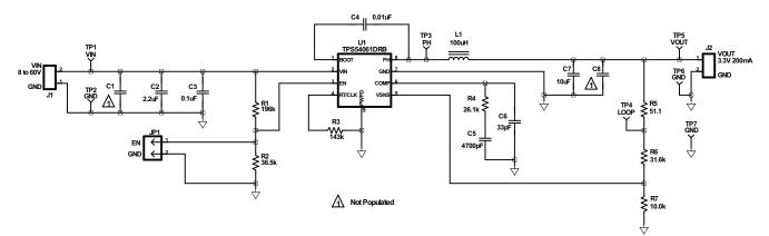
Figure 21. TPS54061EVM-142 Schematic
