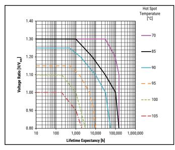
Notes:  $T_{HS} = T_{AMB} + \Delta T$   $\Delta T = ESR * I_{rms}^2 * Rth$  $I_{rms}$  should be limited to values granting  $\Delta T \le 30^{\circ}C$
