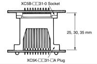
Corresponding to a stacking height of 25, 30, or 35 mm.
