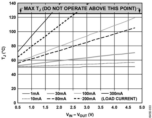
Figure 37. 100 mm<sup>2</sup> of PCB Copper, T<sub>A</sub> = 50°C
