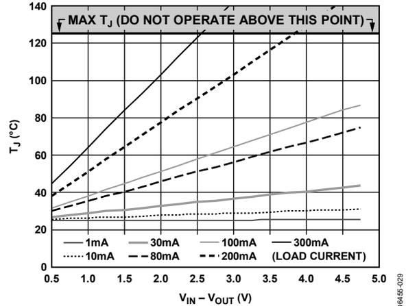
Figure 33. 500 mm<sup>2</sup> of PCB Copper,  $T_A = 25^\circ\text{C}$
