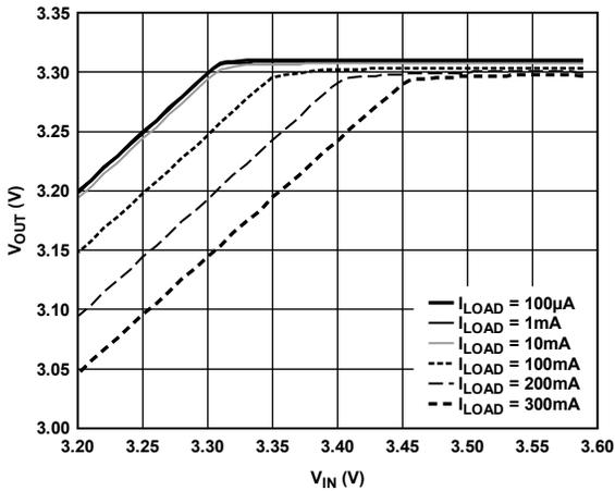
Figure 16. Output Voltage vs. Input Voltage (in Dropout)
