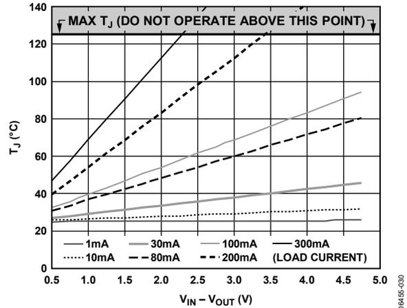
Figure 34. 100 mm<sup>2</sup> of PCB Copper,  $T_A = 25^\circ\text{C}$
