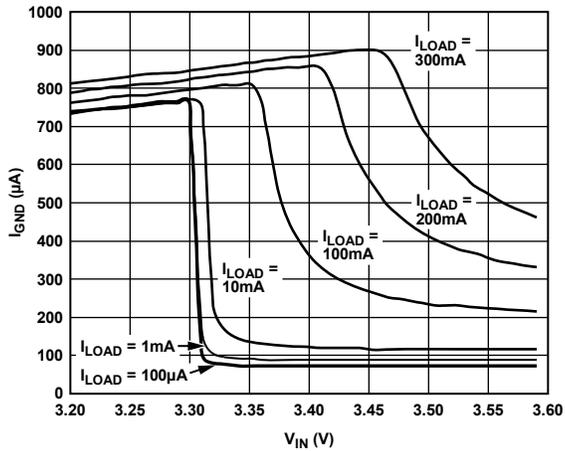
Figure 17. Ground Current vs. Input Voltage (in Dropout)
