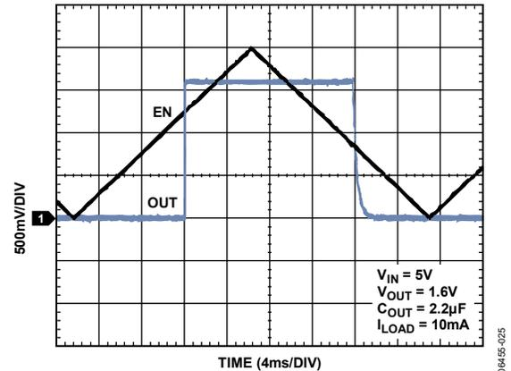
Figure 29. ADP1712 Adjustable Typical EN Pin Operation
