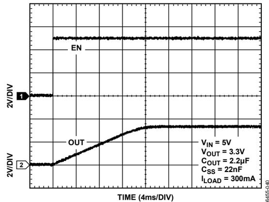
Figure 26. OUT Ramp-Up with External Soft-Start Capacitor
