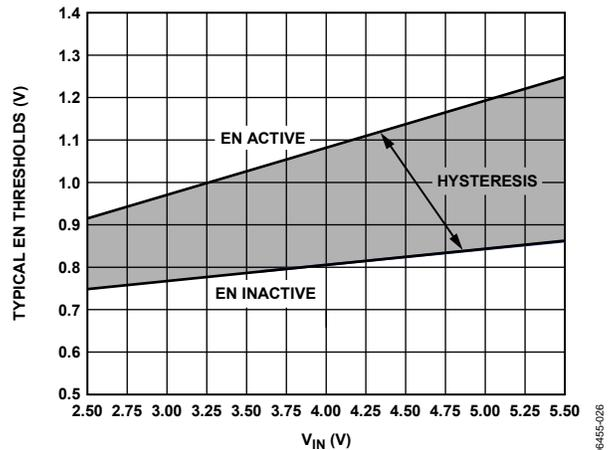
Figure 30. Typical EN Pin Thresholds vs. Input Voltage
