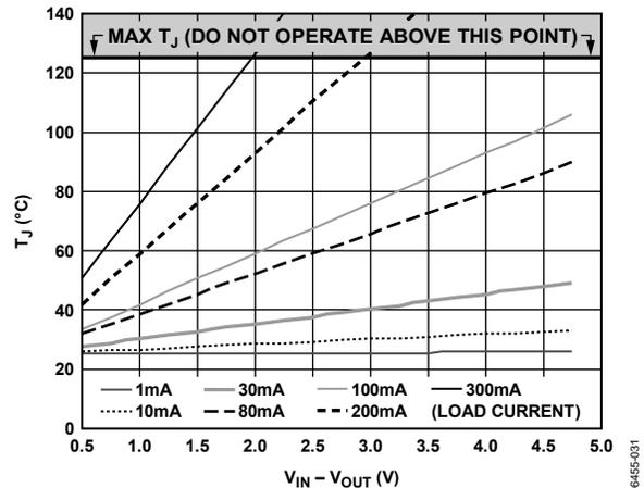
Figure 35. 0 mm<sup>2</sup> of PCB Copper,  $T_A = 25^\circ\text{C}$
