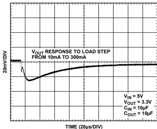
Figure 32. Output Transient Response,  $C_{OUT} = 10 \mu\text{F}$
