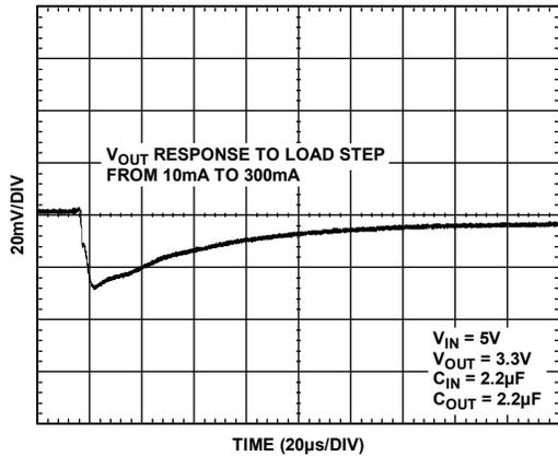
Figure 31. Output Transient Response,  $C_{OUT} = 2.2 \mu\text{F}$
