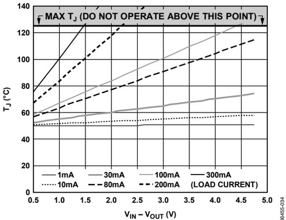
Figure 38. 0 mm<sup>2</sup> of PCB Copper, T<sub>A</sub> = 50°C
