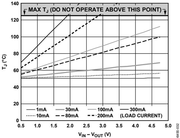
Figure 36. 500 mm<sup>2</sup> of PCB Copper, T<sub>A</sub> = 50°C
