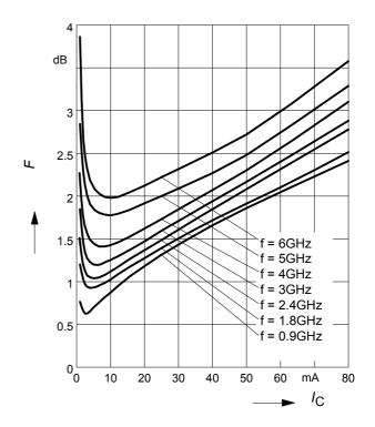
Noise figure F = f(f) $V_{CE} = 2V, Z_S = Z_{Sopt}$
