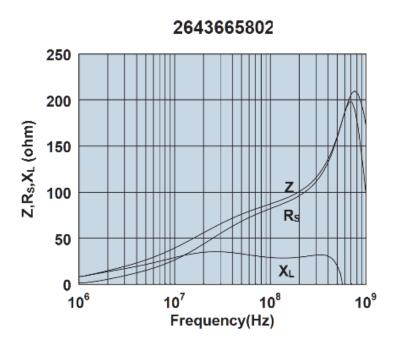
Impedance, reactance, and resistance vs. frequency.
