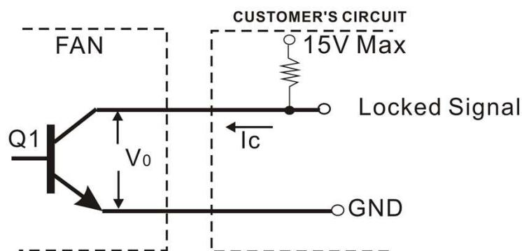
\*Transistor Q1 at "ON" position
