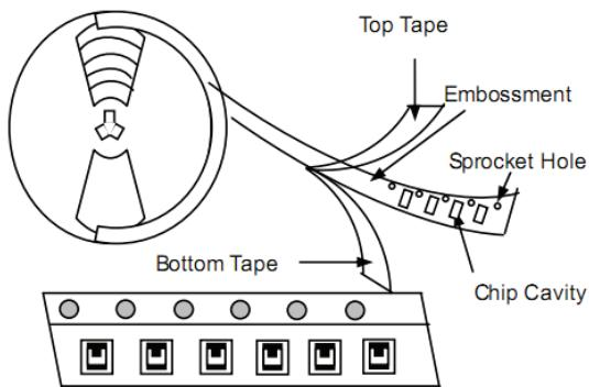
Note: The sprocket holes are to the right as the tape is pulled toward the user.
