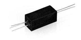
Each Optoisolator in this data sheet contains an infrared Light Emitting Diode (LED) and a NPN silicon Photosensor. The **OPI120** has an 890 nm Light Emitting Diode (LED) and NPN phototransistor sensor, whereas the **OP123** has a 890 nm LED and a photodarlington sensor. The devices are sealed in a precast opaque housing with a optically transmissive path between the LED and the photosensor.
