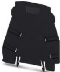
Separating plate, 2 mm thick, required at the start and end of a PLC terminal strip. Furthermore, it is used for: visual separation of groups, safe isolation of different voltages of neighboring PLC relays in acc. with DIN VDE 0106-101, isolation
