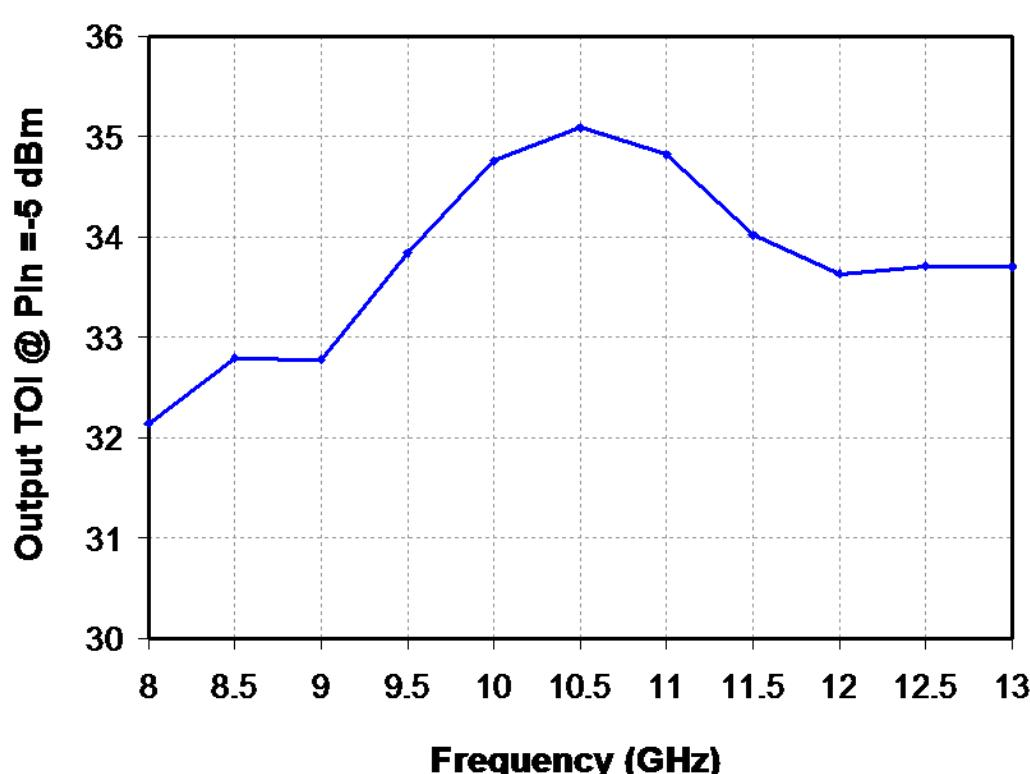
**Typical Fixtured Performance**Bias Conditions:  $V_d = 9V$ ,  $I_{dQ} = 225mA$
