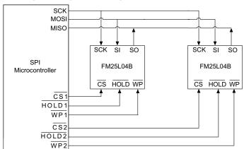
Figure 3. System Configuration with SPI port
