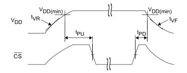
$<sup>\</sup>label{eq:Note} \textbf{13. Slope measured at any point on $V_{DD}$ waveform.}$
