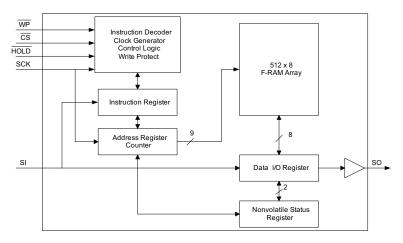
Errata: The Write Enable Latch (WEL) bit in the Status Register of FM25L04B part doesn't clear after executing the memory write (WRITE) operation at memory location(s) from 0x100 to 0x1FF. For more information, see Errata on page 20. Details include errata trigger conditions, scope of impact, available workarounds, and silicon revision applicability.
