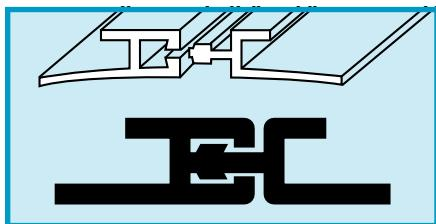
Loc-Trac® provides an effective closure that is ideal for use where the assembly will be subjected to random flexing.
