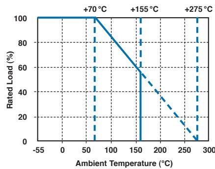
For resistors operated in ambient temperatures above 70°C, power rating must be derated in accordance with this curve.
