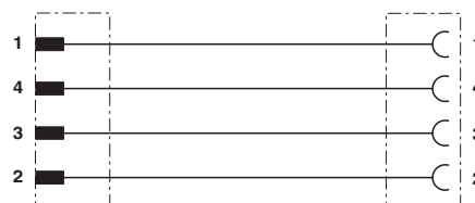
Contact assignment of the M12 plug and the M12 socket
