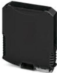
Complete housing, length: 99 mm, with vents, Complete housing, Cross connection: DIN rail bus connector, color: black, width: 22.5 mm, height: 114.5 mm, number of positions cross connector: 5
