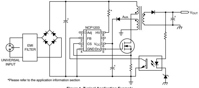
Figure 1. Typical Application Example
