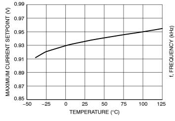
Figure 11. Maximum Current Setpoint versus Temperature
