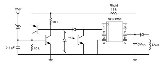
Figure 20. Two Bipolars Ensure a Total Latch-Off of the SMPS in Presence of an OVP
