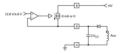
Figure 13. The Current Source Brings V<sub>CC</sub> Above 12.8 V and then Turns Off
