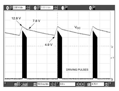
Figure 15. Typical Waveforms in Short Circuit Conditions
