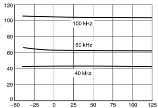
Figure 12. Frequency versus Temperature
