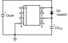
Figure 23. or a diode forces V<sub>CC</sub> to reach UVLOlow sooner
