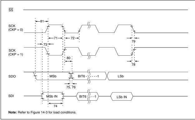
FIGURE 14-12: SPI SLAVE MODE TIMING (CKE = 0)
