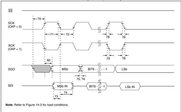
FIGURE 14-11: SPI MASTER MODE TIMING (CKE = 1, SMP = 1)
