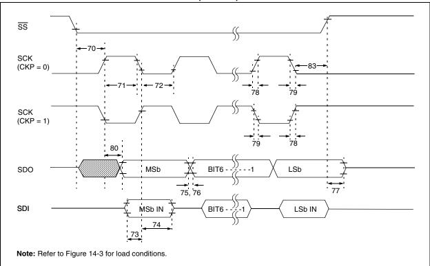
FIGURE 14-13: SPI SLAVE MODE TIMING (CKE = 1)
