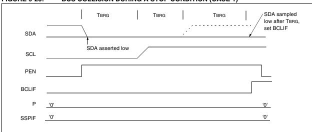
FIGURE 9-26: BUS COLLISION DURING A STOP CONDITION (CASE 2)
