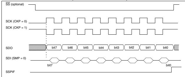
FIGURE 9-4: SPI MODE TIMING (SLAVE MODE WITH CKE = 1)
