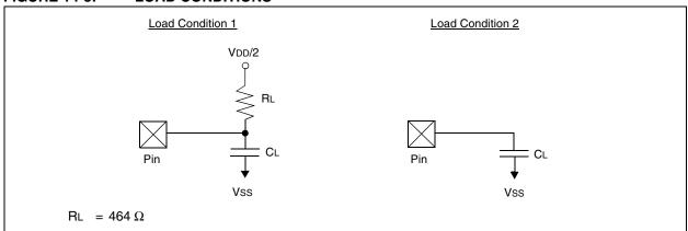
CL = 50 pF for all pins except OSC2, but including PORTD and PORTE outputs as ports 15 pF for OSC2 output
