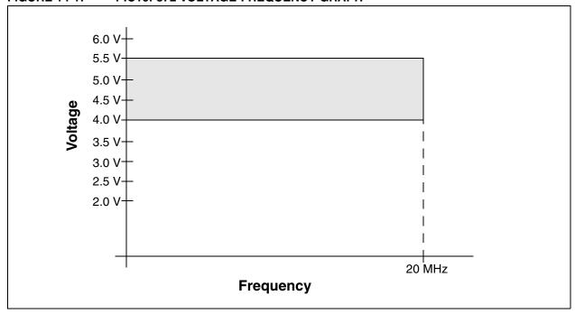
FIGURE 14-2: PIC16LF872 VOLTAGE-FREQUENCY GRAPH
