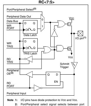
FIGURE 4-6: PORTC BLOCK DIAGRAM (PERIPHERAL OUTPUT
