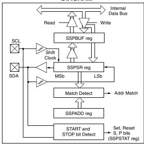
Two pins are used for data transfer. These are the SCL pin, which is the clock, and the SDA pin, which is the data. The SDA and SCL pins are automatically configured when the I<sup>2</sup>C mode is enabled. The SSP module functions are enabled by setting SSP Enable bit SSPEN (SSPCON<5>).
