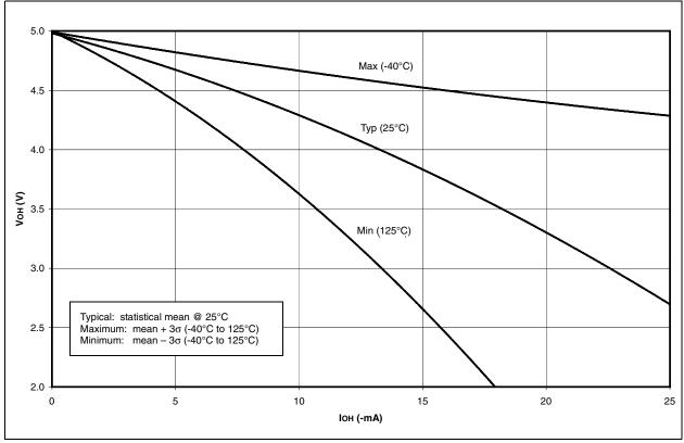
3.0 Max (-40°C) Typical: statistical mean @ 25°C Maximum: mean +  $3\sigma$  (-40°C to 125°C) Minimum: mean -  $3\sigma$  (-40°C to 125°C) 2.5 Typ (25°C) 2.0 Min (125°C) **()** нол 1.0 0.5 0.0 5 10 15 20 25 0 IOH (-mA)
