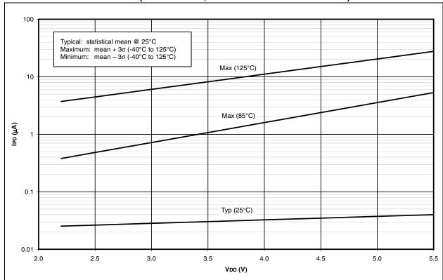
FIGURE 15-11: Albor vs. VDD OVER TEMPERATURE
