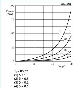
Fig. 10. Average reverse power dissipation as a function of reverse voltage; typical values
