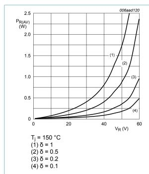
Fig. 8. Average reverse power dissipation as a function of reverse voltage; typical values
