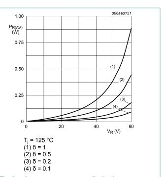
Fig. 9. Average reverse power dissipation as a function of reverse voltage; typical values
