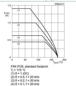
Fig. 11. Average forward current as a function of ambient temperature; typical values
