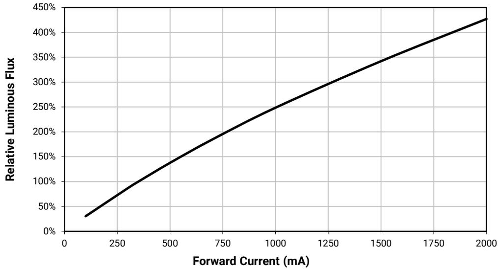
**RELATIVE FLUX VS. CURRENT - STANDARD ( $T_j = 85\text{ }^\circ\text{C}$ )**
