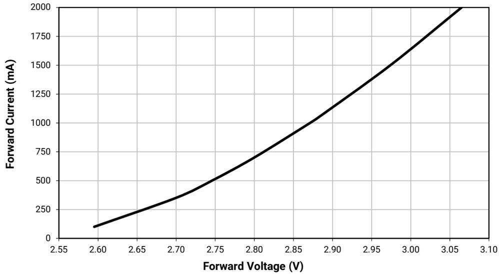
**ELECTRICAL CHARACTERISTICS - STANDARD ( $T_j = 85\text{ }^\circ\text{C}$ )**
