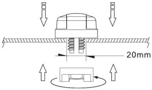
Recommended torque for Mounting is 24.5N·m Maximum torque for mounting is 29.4N·m
