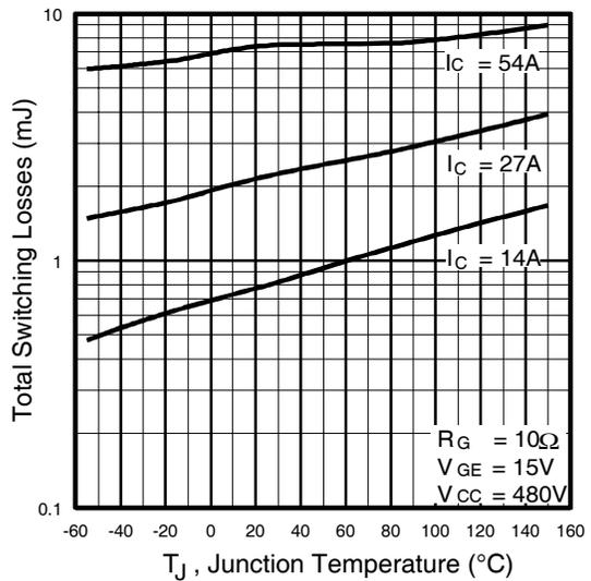
**Fig. 10 - Typical Switching Losses vs. Junction Temperature**
