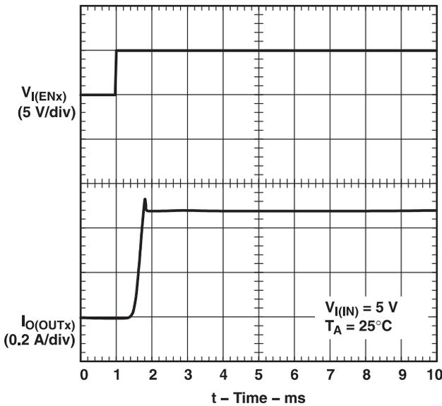
Figure 6. TPS2090, Short-Circuit Current, Device Enabled Into Short
