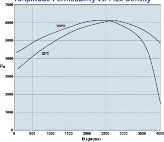
Measured on an 18/10/6mm toroid at 10kHz.
