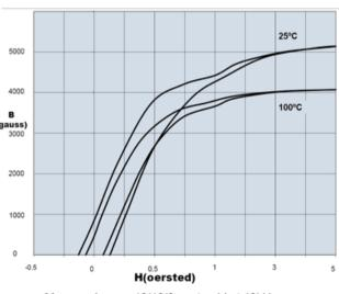
Measured on an 18/10/6mm toroid at 10kHz.
