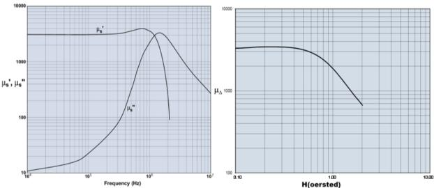
Measured on an 18/10/6mm toroid using HP 4284A and HP4291A.
