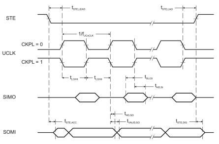
Figure 5-18. SPI Slave Mode, CKPH = 0
