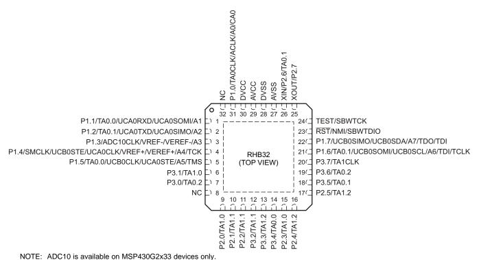
Figure 4-3. 32-Pin RHB Package (Top View), MSP430G2x03 and MSP430G2x33
