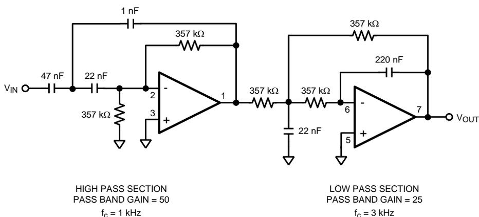
**Figure 1. High Gain Band Pass Filter**
