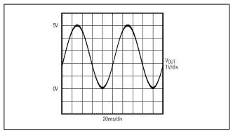
Figure 4. Rail-to-Rail Output Operation
