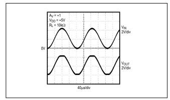
Figure 3. Overdriven Input Showing No Phase Reversal
