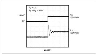
Figure 2a. Pulse Response with No Feed-Forward Compensation
