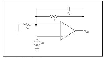
Figure 1. Adding Feed-Forward Compensation
